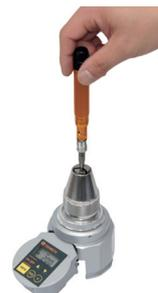
BMRD torque checking with BTGE-G.
